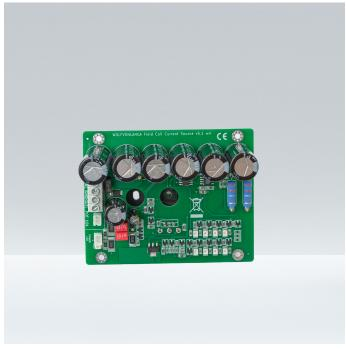
WVL FCCS-5.1 UHQ Field-Coil-Current-Source Recommended Power Supply Module Current adjustable from 1.4 to 3.5ADC High-Quality-Transformer needed
